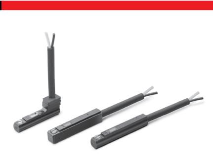
The reed switch that has a mechanical switching element, is suitable for voltages, AC and DC up to 110 V. Proximity switches mod. CSC are suitable for gripper mod. CGL. The proximity switches are impregnated in a sealed isolating cover. These sensors are designed to fit into the grooves provided in the profile barrel of the grippers.
