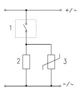
There is no protection on the Reed sensors on the inductive load, therefore it is advisable to use electric circuits with protection against the voltage spikes: the first for direct current (DC), the second for alternating current (AC).
