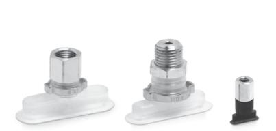
The flat oval suction pads Series VTOF consist of a nipple and rubber part. The nipples are inserted directly into the rubber part.
