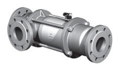
3/2 way valve direct acting pressure range PN 0-16 bar orifice DN 80 mm connection flange
