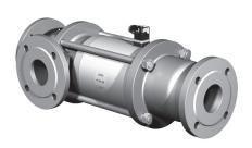
3/2 way valve direct acting pressure range PN 0-16 bar orifice DN 65 mm connection flange
