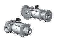
3/2 way valve direct acting pressure range PN 0-40 bar orifice DN 32 mm connection thread/flange
