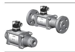
2/2 way valve direct acting pressure range PN 0-100 bar orifice DN 15 mm connection thread/flange
