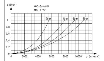
Diagram for lockable manual control valves
