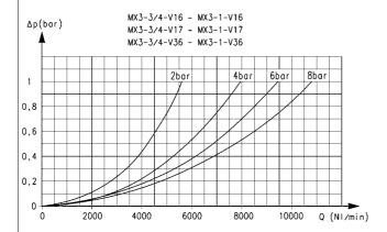
Diagram for electro-pneumatic, servo-pilot or pneumatic control valves
